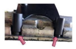
Removal of the back two holes of the original mounting bracket is necessary. This can be removed
